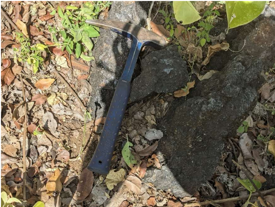
Figure 19: A magnetic ore body in a NW-SE strike direction being surrounded by schists all striking in the same direction as the iron ore. Sample 1 MBOO1 and sample 2 CS001 were collected.
