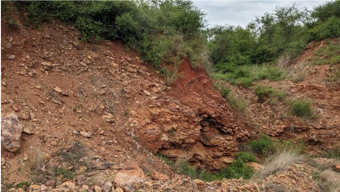
Figure 9: The abandoned pit, elongation of 20 m and wide by 15 m with an overburden soil material about 3 m thick.
